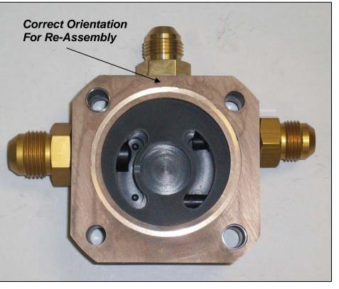
**NOTE:** IF THE BRONZE SECTION IS IMPROPERLY INSTALLED (i.e. INCORRECT ORIENTATION), THE PUMP'S ROTATION HAS BEEN REVERSED AND NO FUEL FLOW WILL BE SEEN AT THE OUTLET FITTING.
